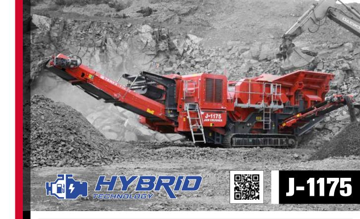
The dual powered Terex Finlay J-1175 jaw crusher offers operators the flexibility to power the plant either by mains electric connection or the onboard genset powerpack configuration. Either power option presents operators with significant power, servicing and maintenance cost savings in direct comparison to a diesel/hydraulic powered plant.
