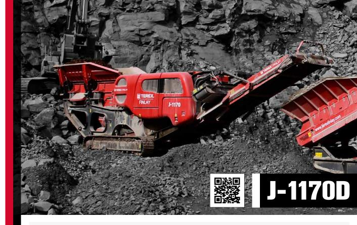
The Terex Finlay J-1170 is a compact and aggressive tracked primary jaw crusher. The heartbeat of the machine is a robust direct driven Terex jaw chamber which provides high capacity with large reduction ratios. The jaw chamber configuration can be set up specifically for quarrying applications or processing construction demolition debris using the hydraulic release chamber option.
