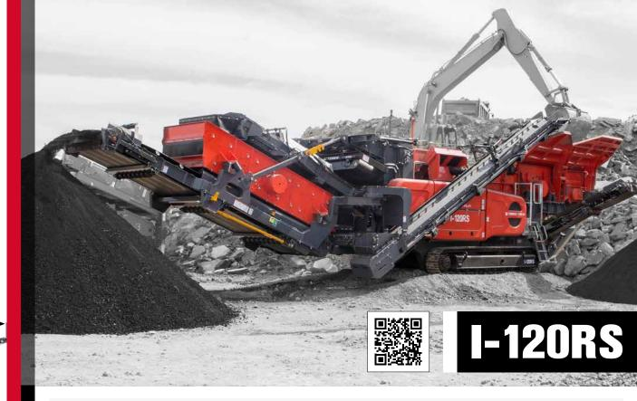
The Terex Finlay I-120RS shapes the future through innovation. This new generation impact crusher with redefined style and advanced technological design gives improved material flow and production capabilities in quarrying, mining, demolition and recycling applications. Incorporating the Terex® CR038 impact chamber with direct drive and advanced electronic control system the machine provides operators with high material reduction ratios and produces a consistent product shape.
