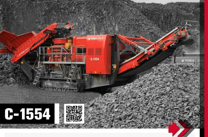
The Terex® Finlay C-1554 is the ultimate mobile solution for any aggregates producer or contractor looking for a high output capacity machine that provides large reduction ratios and an excellent cubical shape.
