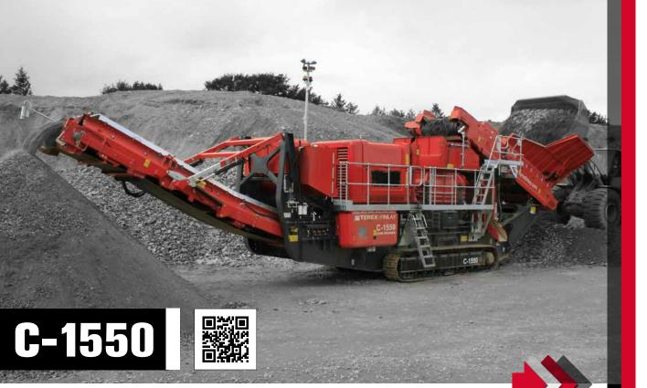
The Terex® Finlay C-1550 is a high capacity and aggressive cone crusher for the surface ore mining and aggregate industries. This efficient and productive machine incorporates the proven Terex® 1300 cone crusher with direct variable clutch drive, automatic tramp relief and hydraulic closed side setting (CSS) adjustment.
