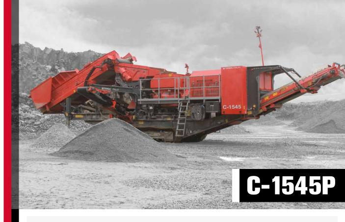
The Terex® Finlay C-1545P incorporates the Terex 1150 cone crusher driven through by direct clutch drive with variable speed, automatic tramp relief and hydraulic closed side setting (CSS) adjustment.
