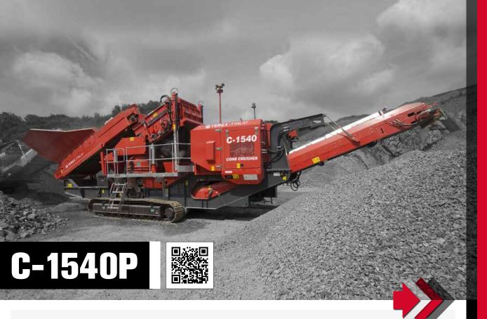
The Terex Finlay C-1540P tracked mobile cone crusher has a proven pedigree in aggregate and ore surface mining applications. This efficient and productive machine incorporates the proven Terex® 1000 cone crusher with direct variable hydrostatic drive, automatic tramp relief and hydraulic closed side setting (CSS) adjustment.
