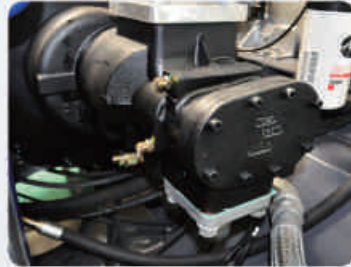
Compressor Air Volume [SD112E: GHH CF75G] 5.7m 3 /min [SD142E: GHH CF90G] 8.7m 3 /min
