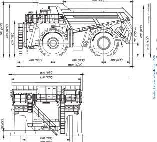
\*Overall dimensions are specified for basic kitting-up of the dump truck
