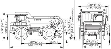
\*Overall dimensions are specified for dump truck with standard options
