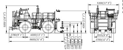
\*Overall dimensions are specified for basic kitting-up of the recovery tractor
