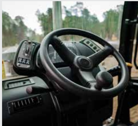
Tilt steering column. Ergonomic steering wheel that does not require significant efforts from the operator when maneuvering. The wheel has a wheel spinner to help make steering with one hand less difficult & faster.
