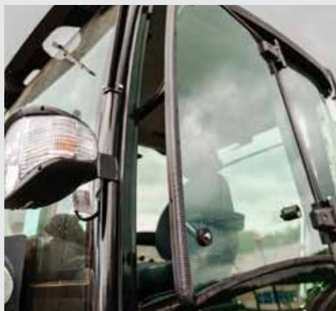
The upper parts of the doors can be fully opened and locked for better ventilation.
