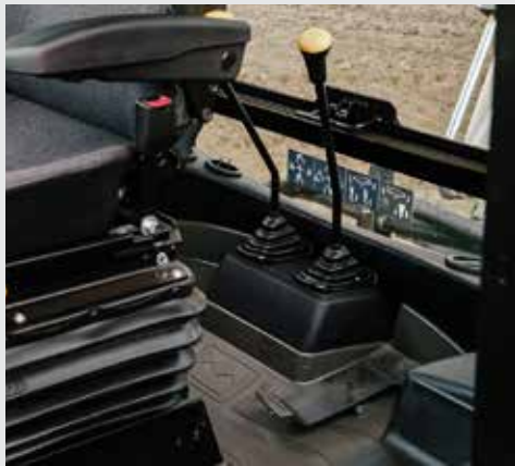
Ergonomic pedal to control the breaker and telescopic stick. It substantially reduces the operator's fatigue.
