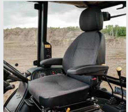
Comfortable adjustable high-back operator's seat with armrests, headrest and retractable seat belt.
