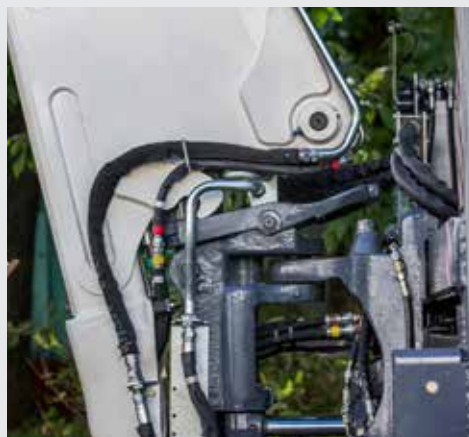
Double-pin boom lock for securing the backhoe boom for transport. This function does not require exit of the operator since it is remotely activated from the operator's cab.
