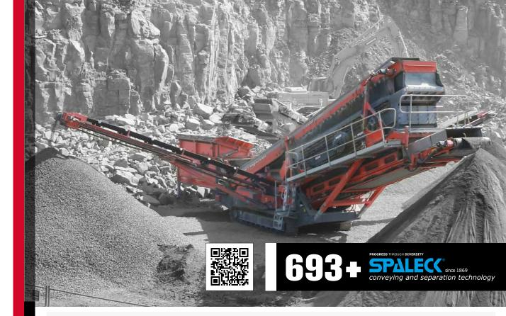
The Terex Finlay 693+ Spaleck is the ultimate in mobile fine screening and separation technology. At the heart of the plant is an innovative 2-deck German designed and constructed high performance aggressive screenbox with state of the art flip flow technology on both the top and bottom decks.
